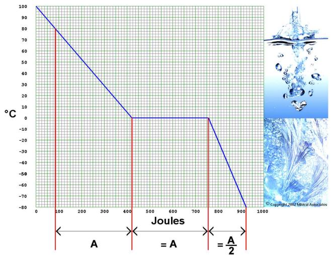
To reduce the temperature of ice from 0°C to -80°C requires the removal of less than half the energy than it did to either remove the Latent Heat from the water or to reduce the temperature of the water by 80 degrees.
